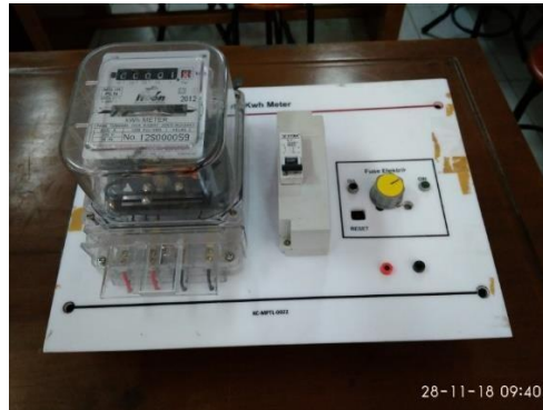
Gambar 4. Panel KWH Meter dan Voltage Regulator
