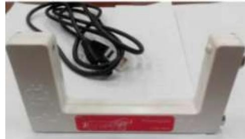
**Gambar 3.** Sensor *Photogate*
