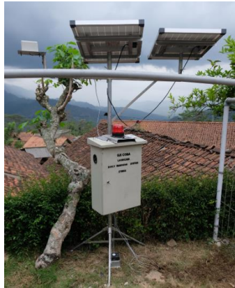
Gambar 4. On site Alat peringatan dini longsor
