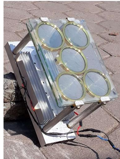
Gambar 3. Prototype Generator Termoelektrik
